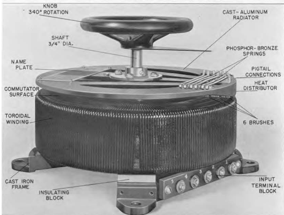
FIGURE 2. TYPE 50-B Variac with cover removed.
